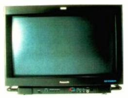
resolution of greater than 1000 lines due to a temperature compensate shadow mask.
