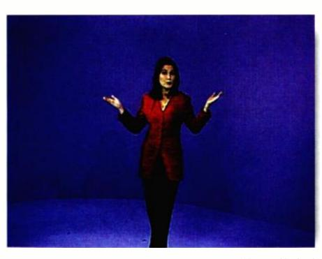
The basic bluescreen backdrop of the set remains in place while a multitude of virtual environments can keyed upon it, benefiting a station's bottom line through reduced set construction and removal costs.
