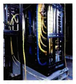
Some of the wiring that goes into a completed RIB assembly can be seen. In the lower right is one of the wedges used to pin the back of the RIB in the shipping container. Also note that the racks sit slightly off the steel floor, held up by the cable shock-mounts.
