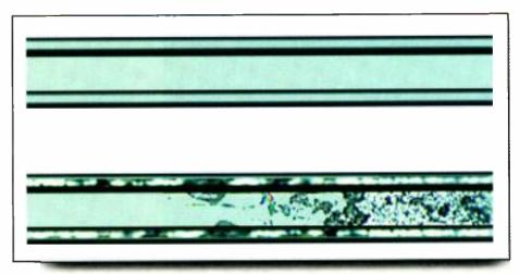
Microscopic photos of a portion of a digital video tape head. The photo on top shows a clean head, while the bottom photo shows a good view of accumulated debris. Photo courtesy of Sony.
