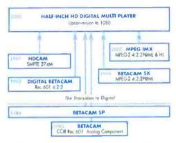
The new Half-Inch HD Digital Multi Player establishes a crucial bridge between SDTV and HDTV. It plays back Digital Betacam. Betacam SX, Betacam and Betacam SP tapes and upconverts each to the 1080-line or 720P formats. while maintaining compatibility with existing HDCAM tapes.
