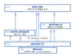
The new Half-Inch MPEG IMX VTR will play back all of the SDTV Betacam formats — both digital and analog.
