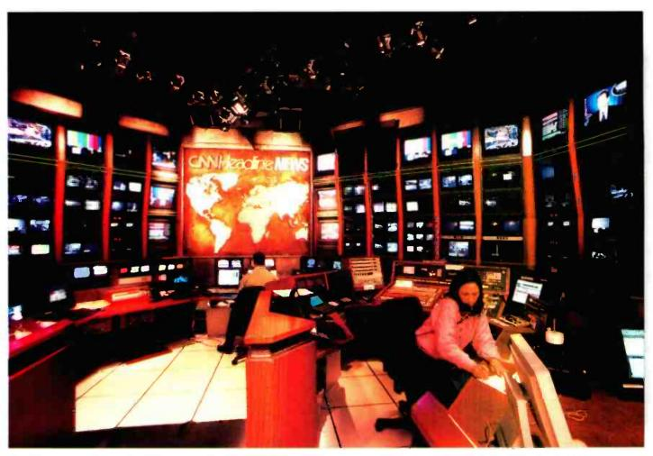
Control room for CNN Headline News. The main technical operating position, shown on the right, uses a GVG 4000 production switcher
